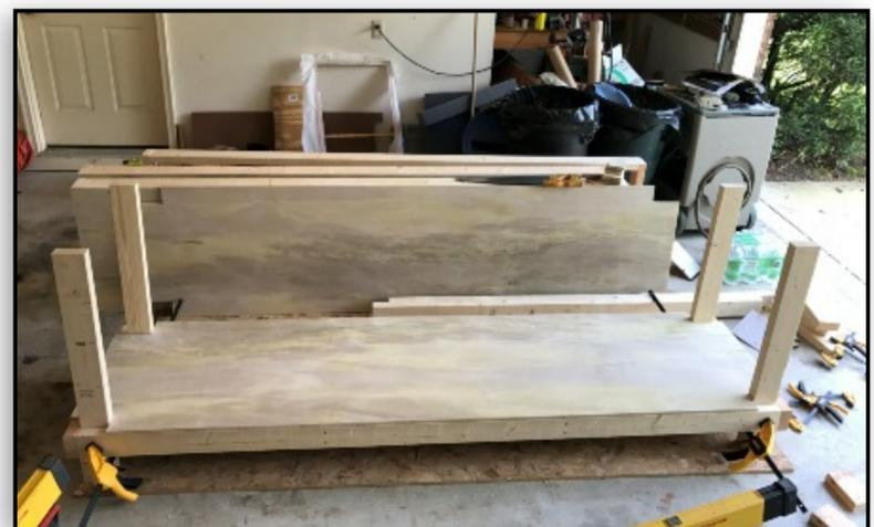
(the one with the cutouts) on the legs. The legs go through the cutouts, the shelf's frame rests on the 4" boards attached to the legs.
